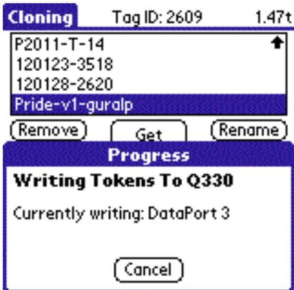
> Then the Q330 configuration must be saved and the unit rebooted
